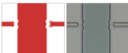
Simulated 2D Resist Contour
