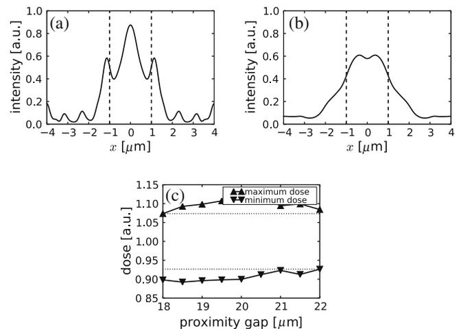
**Fig. 3.** (a) Shows the intensity profile at a proximity gap of 20  $\mu$ m obtained with a mask consisting of 2.9  $\mu$ m lines and a pitch of 8  $\mu$ m using a plane wave as illumination. The intensity profile obtained when using an optimized IFP is shown in (b). The corresponding process window is shown in (c).
