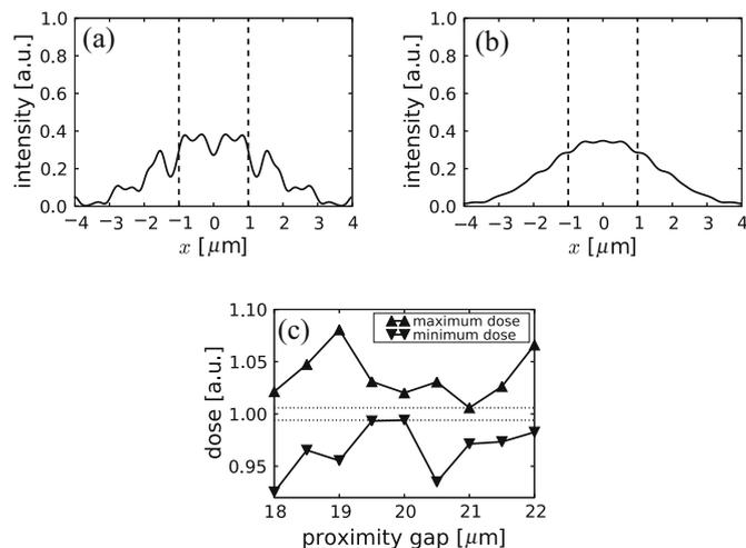
**Fig. 2.** (a) Shows the intensity profile at a proximity gap of 20  $\mu$ m obtained with a mask consisting of 2  $\mu$ m semi-dense lines using a plane wave as illumination. Using an optimized IFP, the intensity profile looks more favorable, as shown in (b). The process window obtained when using the optimized IFP is shown in (c).
